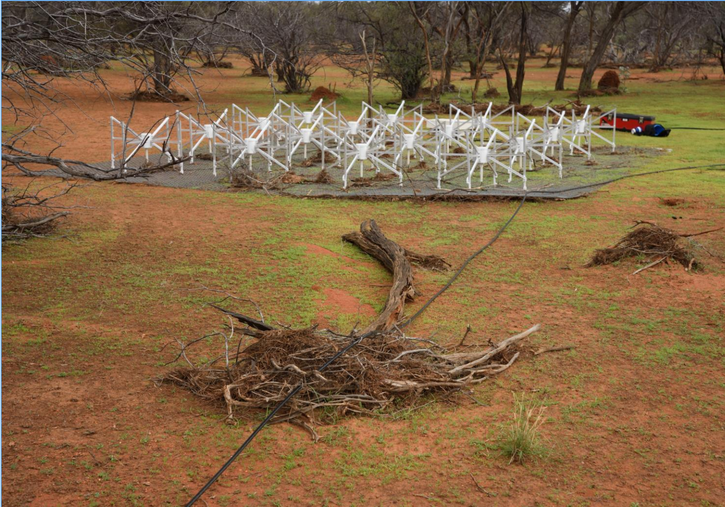
Jan 2018: Long baseline Tile F8 was downstream of a wide creek bed, and suffered substantial damage. Surrounding trees helped to block the tile from some of the debris.
