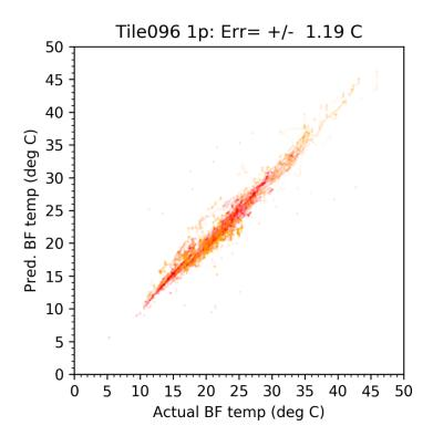
Figure 1: Predicted versus actual beamformer temperatures for Tile096, 2013-2018. Red dots are for measurements before 2017/06/15, orange dots for after that date. Fit parameters used to generate the predicted temperatures are different for the two periods.
