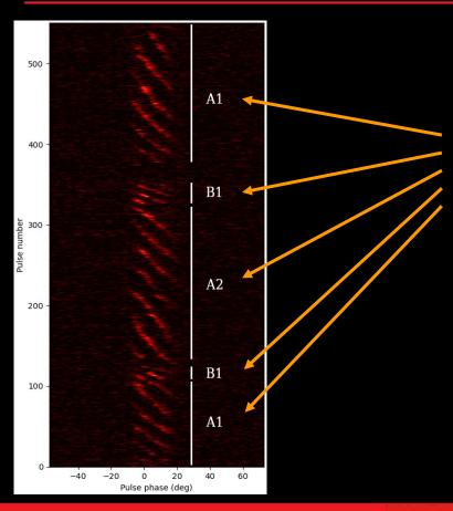
Classification based on how "spread out" the drift bands are (i.e. vertical separation, "P<sub>3</sub>")
